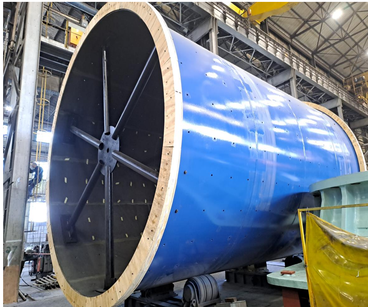
Secondary Mill Shell
